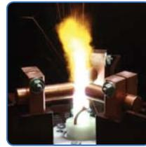
When an arc flash occurs, the arc is diverted by creating a secondary arc fault, not a bolted fault as in crow bar systems.
